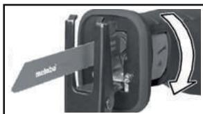
4. Check that the saw blade is securely seated.
