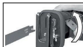
2. Insert the saw blade as far as it will go or remove it (Fig. C).
